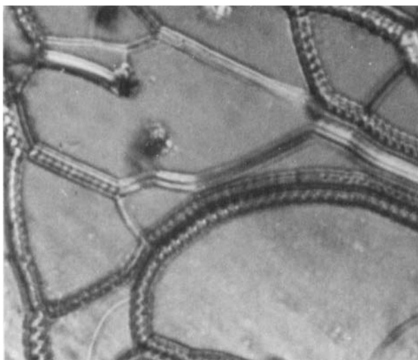
FIGURE 7 Cholesteric texture of a 20:80 mixture of P-6M and P-6 at 200°C (100X).
